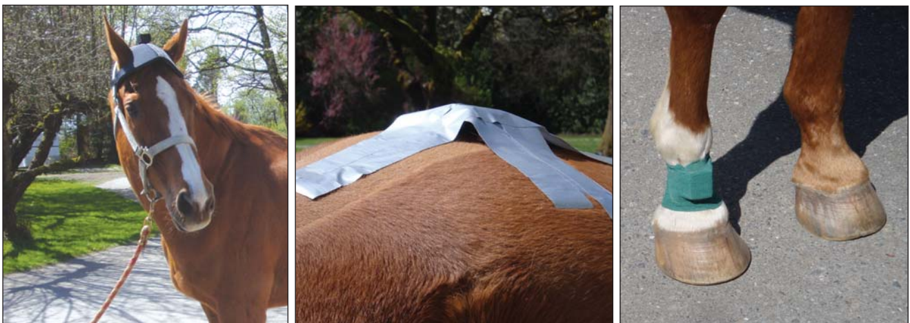
The Lameness Locator™ utilizes the data transmitted from wireless inertial sensors on a horse's head, croup and right front pastern (left to right).
